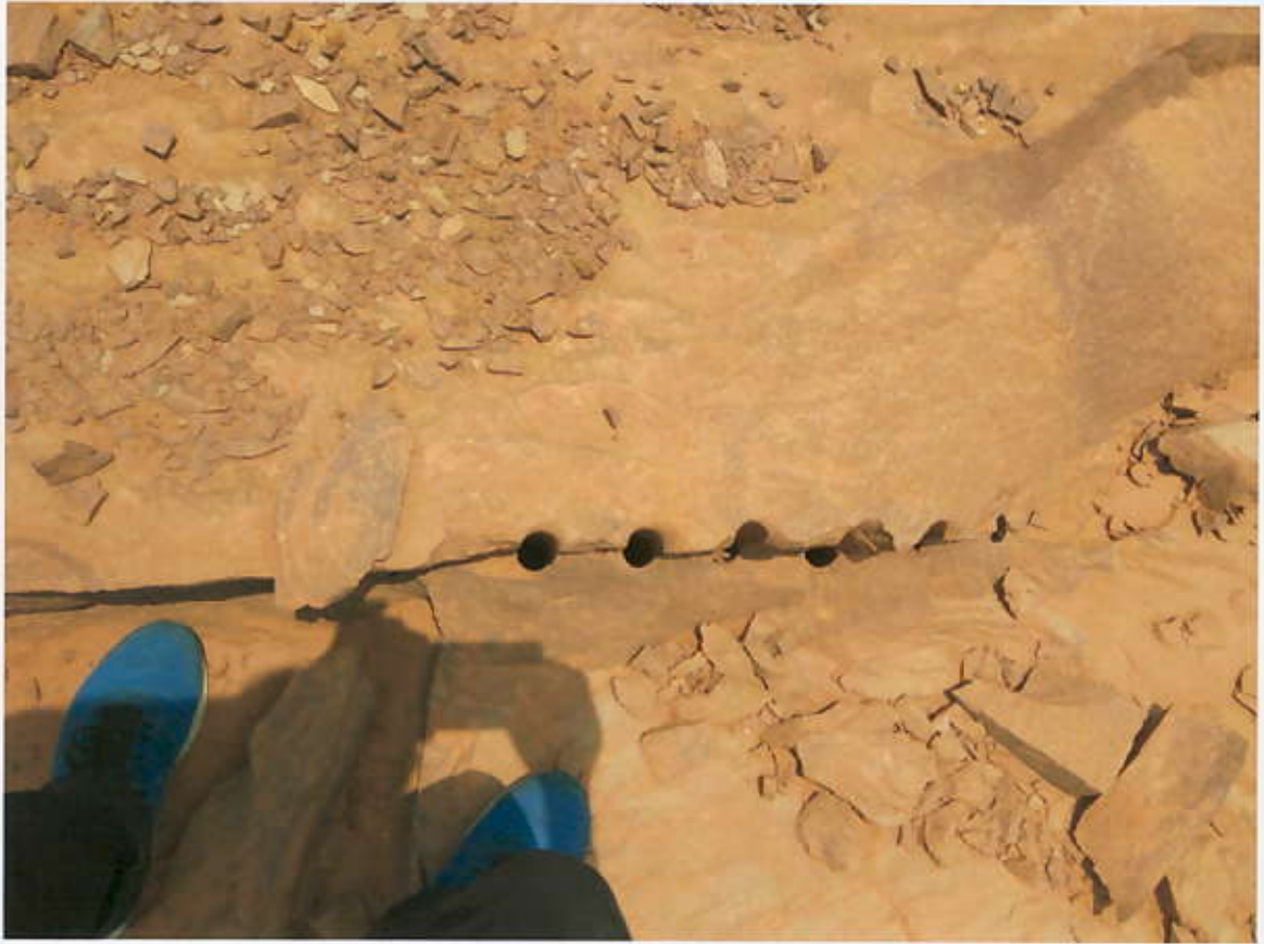
Mining Process, Removal of Farsh Blog ck by making hole
